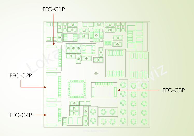
FFC: Flat Flex Connector, Used with flex cable. C#P: Core x to Peripheral, # = 1, 2, 3, 4
